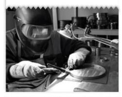
Components are fused together using argon inert gas or aluminium welding.
